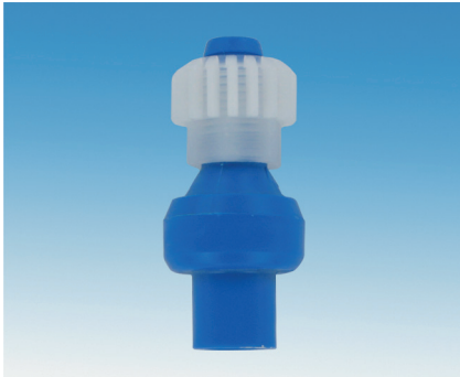
3006.01.20 Filter X-FIX for inline pumps mesh filter, assembly at pump suction side connection: hose inner diameter 10 mm diameter / height: max. 27 / 71 mm
